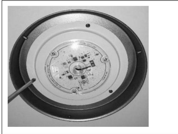
7. Connect two plugs. Connect the wire from fan to LED disc. Attach the LED disc to the center of the light box.
