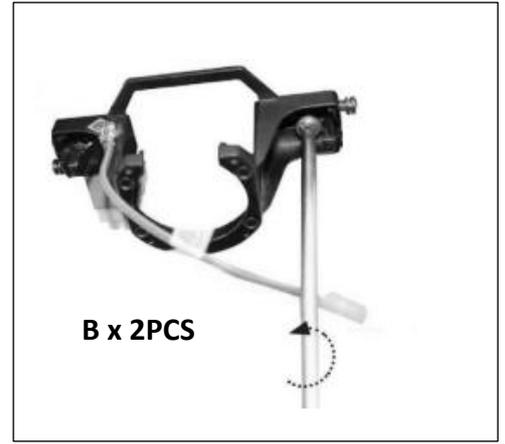
1. Remove the canopy from the mounting bracket, install the mounting bracket to the ceiling. (please ensure the fixing is able to support minimum moving weight of the fan which is 15.8kg=35Lb)
