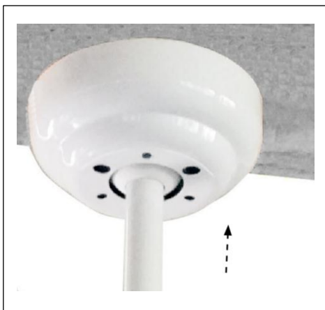
11. Assemble the canopy with the bracket again and using the fixing screws to tighten the canopy, make sure that the canopy is secured and that you have not trapped any wires.
