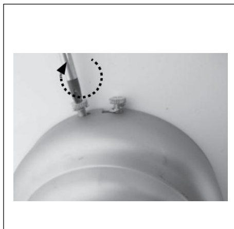
11. Assemble the canopy with the bracket again and using the fixing screws to tighten the canopy, make sure that the canopy is secured and that you have not trapped any wires.
