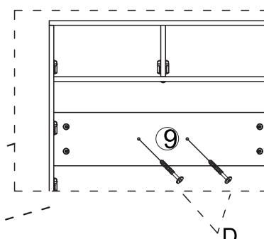
**EN** As shown in the figure, the screw D is passed through the holes of Part 9 to fix the cabinet on the wall.
