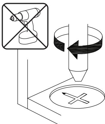
**EN**\_Turn cam lock clockwise to tighten.
