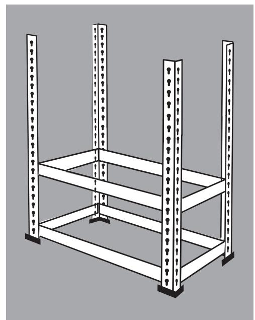
5. Fit long and short shelf supports into the keyhole tracks, using the third and top shelf positions (pic 5).
