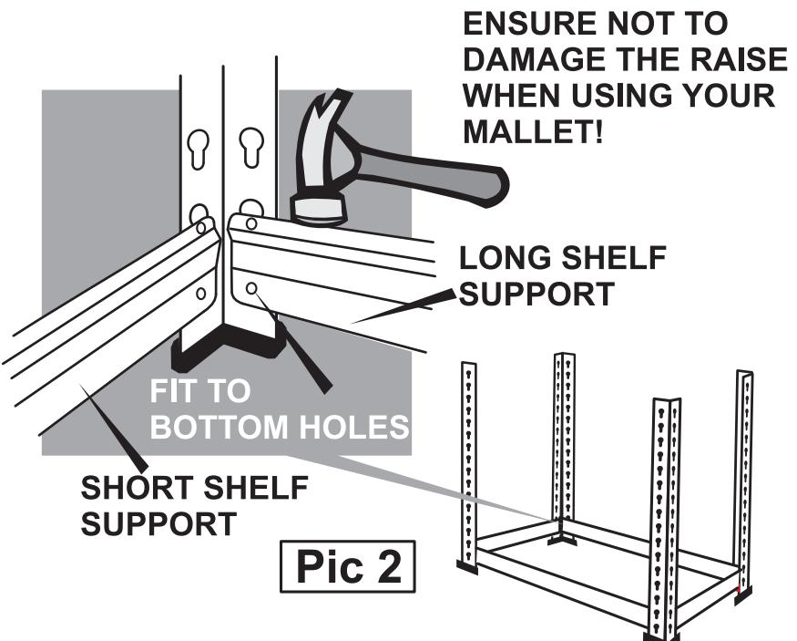
3. Fit long and short shelf supports to your desired position. Do not place these supports into the top two keyholes (pic 3).
