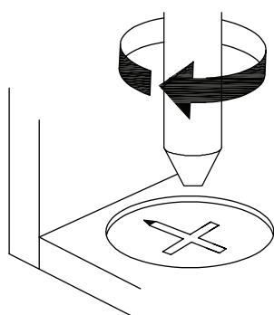
**EN**\_Turn cam lock clockwise to tighten.
