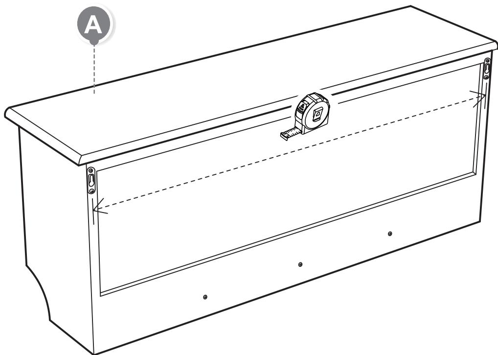
**EN:** Use a tape measure to measure the distance between the centers of the two lifting lugs.
