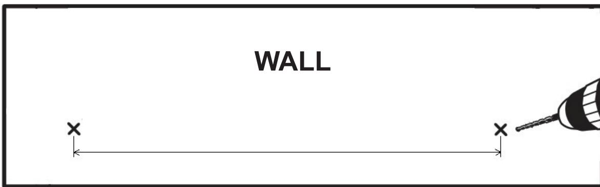
**EN:** Drill the hole with an electric drill, and hammer the wall anchor to the wall in the drilled hole.
