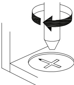
**EN\_**Turn cam lock clockwise to tighten.
