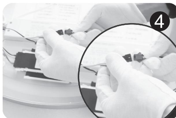
Cut off the connect of touch screen and light strip, take off the connect with yellow red white line and black white color connector
