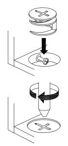
**EN**\_Quickfit head should be in the centre of the cam lock when the two panels are joined.
