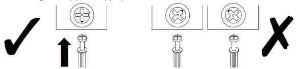
**EN\_CAM LOCK:** When fitting cam lock, ensure starting position is correct before you insert connecting quickfit.
