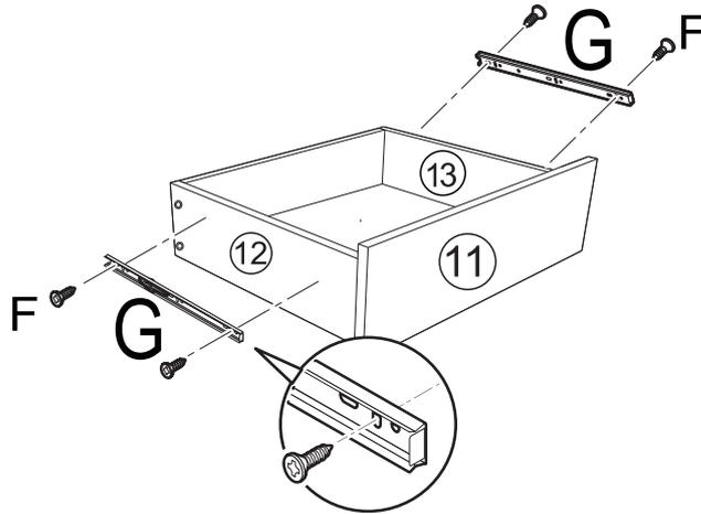
**EN** Please find the exact hole for installation, otherwise it will be misaligned. The screws on the drawer slide must be leveled, otherwise it will affect the smoothness of the drawer.
