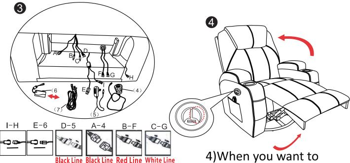
3)Connect the massage, heating, power and transformer supply cable pins. Fit the pins properly in the manner shown in the image.Do not force them, they only have one correct position.
