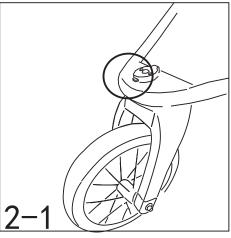
2.Assemble the front wheel: insert the axle of the wheel into the hole **TILL A SOUND "CLICK"** as picture 2-1.
