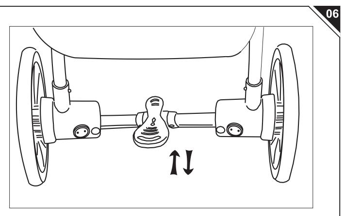
**6**. To step the brake pole down to stop the stroller, and lift it up to release the brake.
