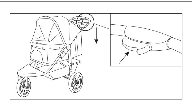
8. Fold the stroller: unzip the canopy window first, then press the folding button as arrow direction to fold the stroller and fasten the folding hook.
