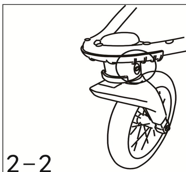
**2.** Assemble the front wheel: insert the axle of the wheel into the hole **TILL A SOUND "CLICK"** as picture 2-1.
