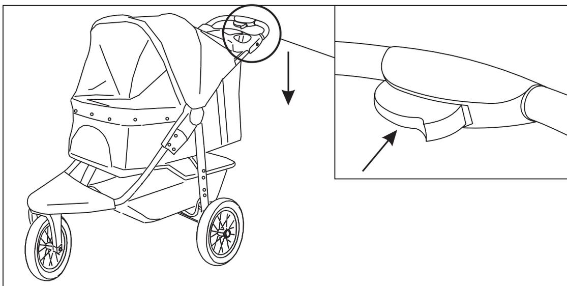
**8. Fold the stroller: unzip the canopy window first, then press the folding button as arrow direction to fold the stroller and fasten the folding hook.**
