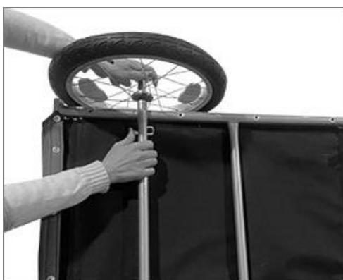
4. Open the cabin, install the roof bar and lock the pin
