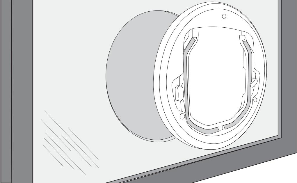
**EN** Install exterior frame into hole and slide interior frame over top to required fit.
