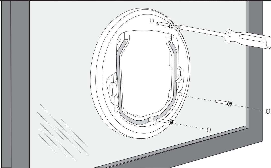
**EN** Ensure door is level and secure using the 3 enclosed screws and plastic caps
