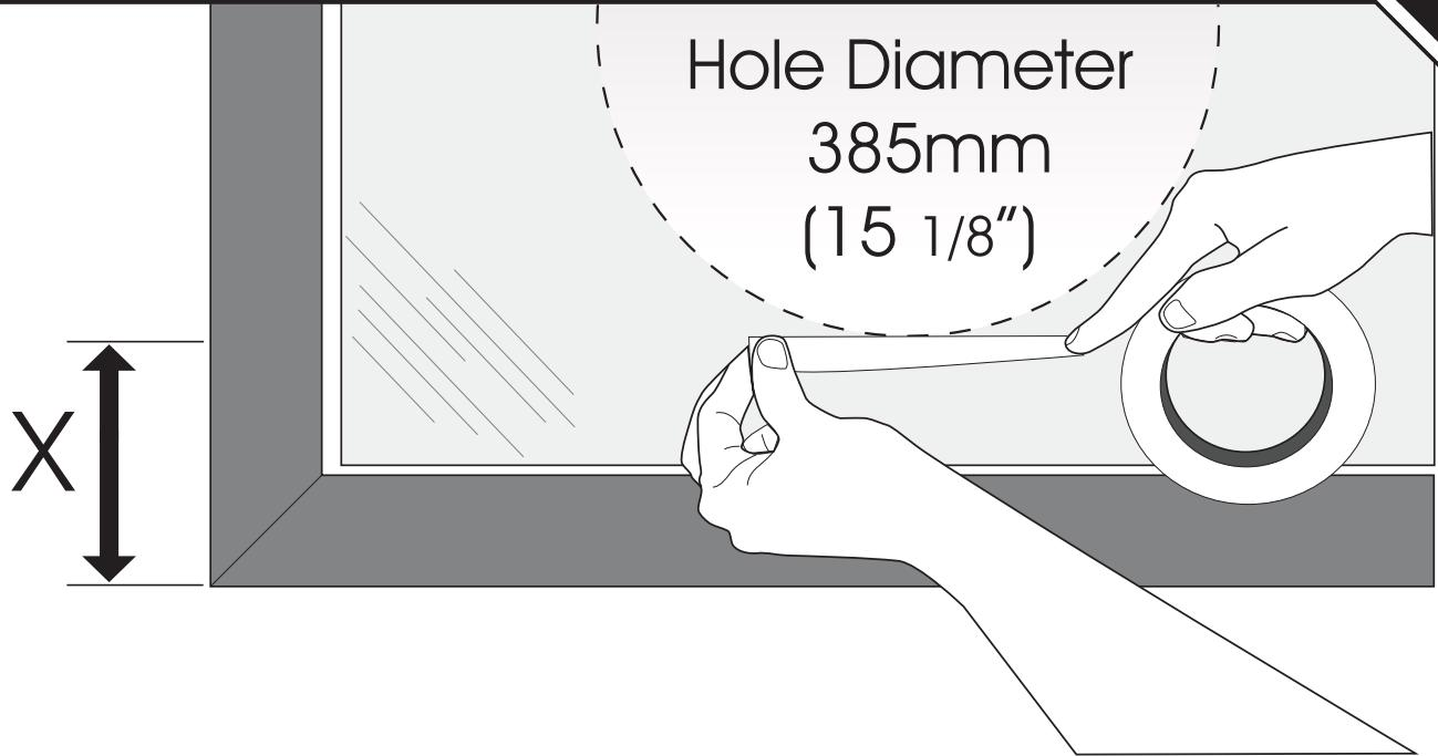
**EN** Mark height (x) on glass panel with tape or similar, and cut required hole out above.
