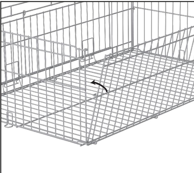
**EN\_Weave** the Back Panel and the Side Panels together using the “J” Shaped Wire hooks.
