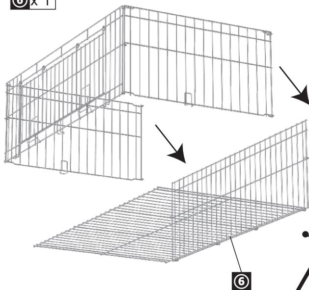
**EN\_Connect the Upper Top and Back Panel to the connected Upper Section Front and Upper Section Side panels by placing the Upper Top and Back Panel onto a flat surface and connecting the back panel to the Side Panels using the "J" shaped wire hooks.**
