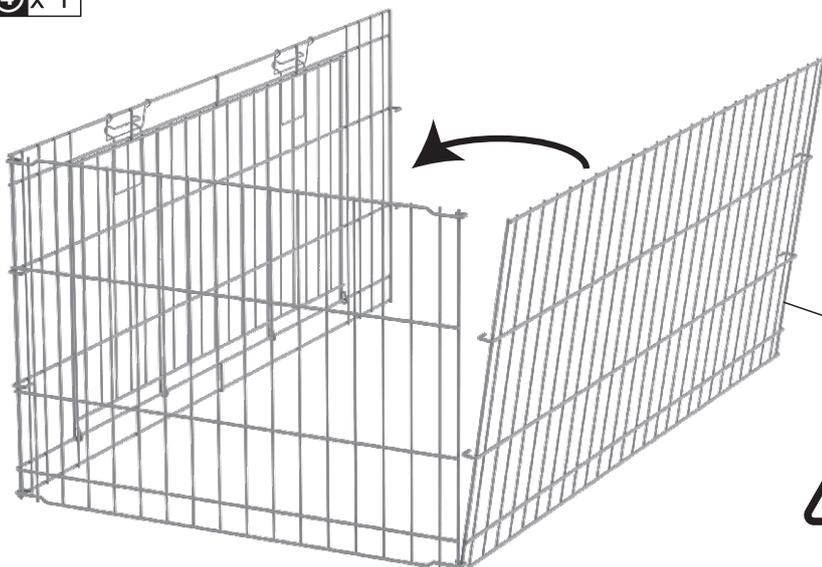
**EN\_Connect** the Lower Section Back Wire Panel to the Lower Section Side Panel using the “J” Shaped wire hooks.
