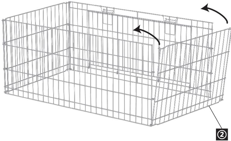
**EN** Connect the remaining Lower Section Side Panel to the Lower Section Front and Back Wire Panels using the “J” shaped wire hooks.
