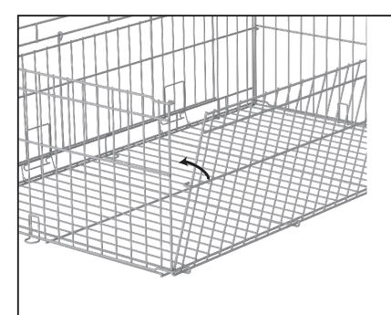
Weave the Back Panel and the Side Panels together using the "J" Shaped Wire hooks.
