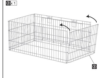
Connect the remaining Lower Section Side Panel to the Lower Section Front and Back Wire Panels using the "J" shaped wire hooks.
