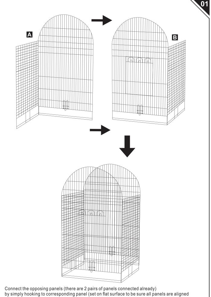
by simply hooking to corresponding panel (set on flat surface to be sure all panels are aligned correctly).Once hooked together, crimp hooked end tight [use a long nose pliers (NOT INCLUDED) over a cloth to prevent scratching]
