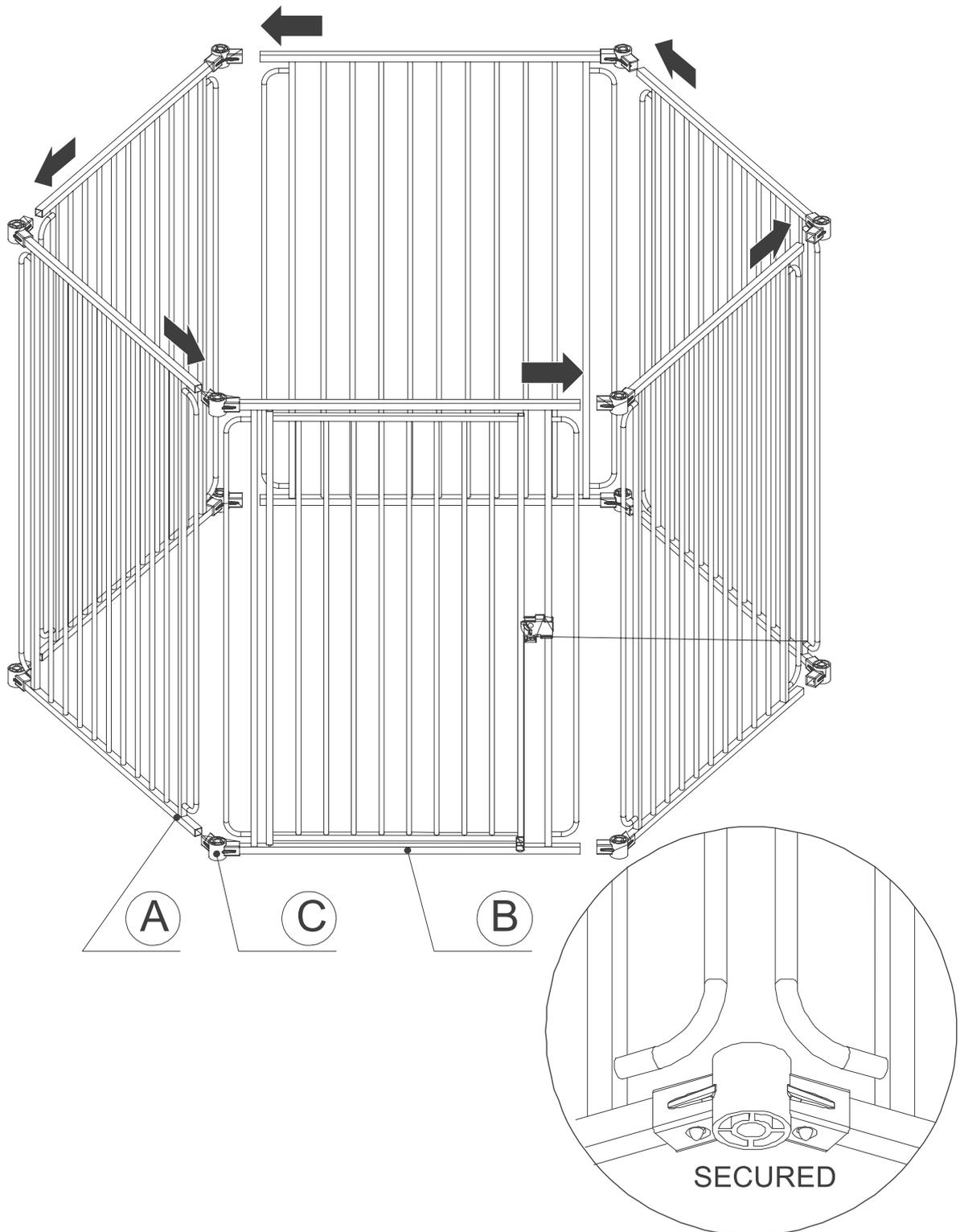
**NOTE:** Make sure that the spring pins are secured into the opposing holes.
