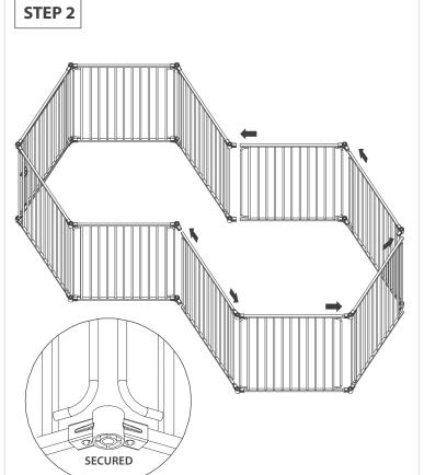
**NOTE:** Make sure that the spring pins are secured into the opposing holes.
