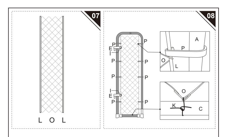
Install the chain-link mesh onto the gate frame. Then insert the two round rod into the edges of the chain-link mesh, and then use 4 pairs of hooks to fix the round rods and tube. Finally, use the bind-wire fo fix the chain-ink mesh to the gate frame to make the gate rigid and strong. (Note: loosen the clips on the post to allow adjustment and exact fitment)
