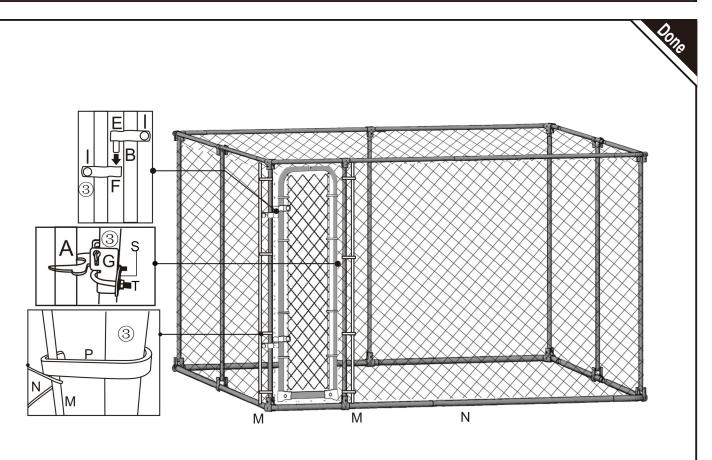
Use the door hinges (and the big set of screws) to fix the door to the frame. Then install the security-lock on the dog run. Tie bind wire to fix the top and bottom of the gate with chain-link mesh and make the gate safe and strong by using the screw gun with the drill to put a self-tapping screw through the pilot holes in the tubes-this also makes the dog run stronger.
