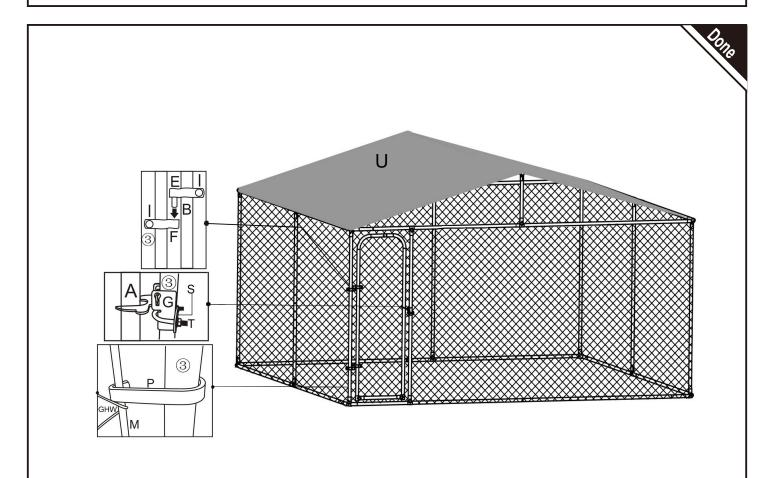
Use the door hinges (and the big set of screws) to fix the door to the frame. Then install the security-lock on the dog run. Tie bind wire to fix the top and bottom of the gate with chain-link mesh and make the gate safe and strong by using the screw gun with the drill to put a self-tapping screw through the pilot holes in the tubes-this also makes the dog run stronger.
