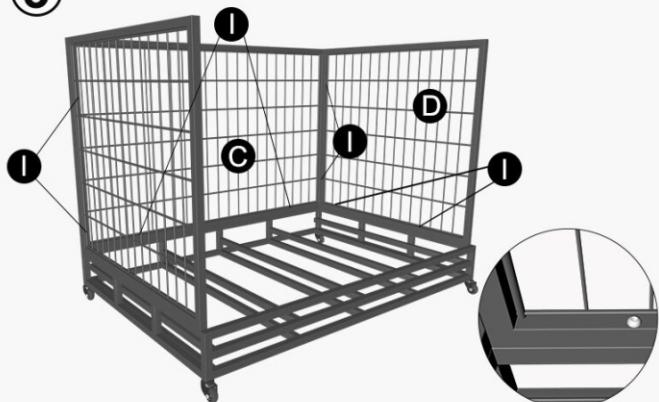
Install the back plate in the same way, and then fixthe back plate and left and right side plates withscrews.
