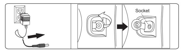
1. to open the charging hole cover. Plug the charger into the charging hole. (charging hole in the rear of the body)
