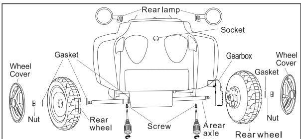
5. Rear tail light installation As shown by the self tapping screws fixed on the vehicle taillight corresponding hole.
