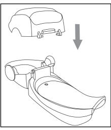
9. The installation of the toolbox Position the cover of the toolbox at the bottom of the trunk seat behind the seat and fasten the two front buckles on the bottom of the trunk seat.
