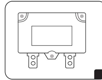
When the vehicle won't work or can not be charged, please check the fuse first and see whether it is burnt out. If the fuse is broken, please change with a new one, there is a spare fuse in the fuse package. The fuse is under the seat.
