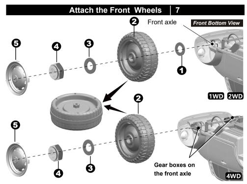
Remove all the parts from the front axle.
