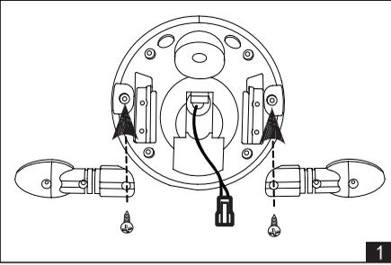
1. Assembling front light according to arrowhead, using 2pcs 4x12 screw to tighten.
