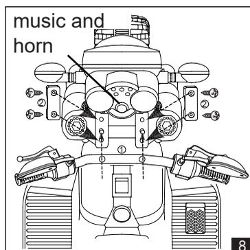
8. Inserting headstock on
