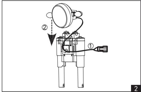
2. Passing light line through front fork(1), putting front light into front fork(2).
