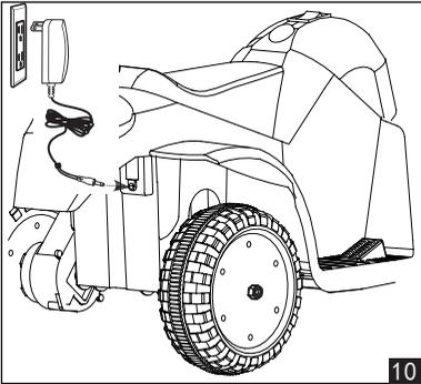
10. Battery charge: please charge tricycle when battery is low. Charging hole is on the left side of the right wheel. Connecting charging hole, then charge(10).
