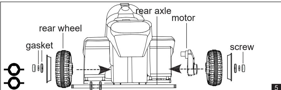
5. Assembling order to rear axle for left side is rear wheel, rear wheel cover, gasket, screw, for right side is motor, rear wheel, rear wheel cover, gasket, screw.
