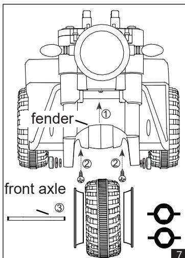
7. Assembling fender(1). Using 2pcs 4x12 screw to tighten(2).
