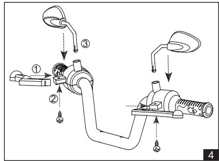
3. using 4pcs 4x12 screw to tighten.
