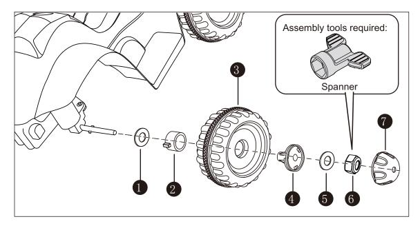
Remove all the parts from the front axle.
