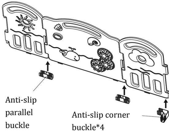
3. Install anti-slip parallel buckle and anti-slip corner buckle:
