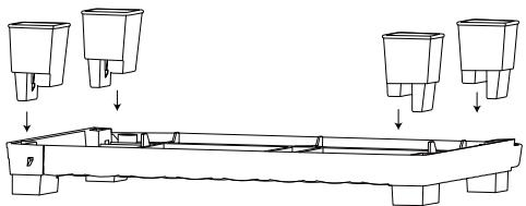
**EN:** Put the scaffold into the bottom hole of the support frame and confirm that it cannot be moved.
