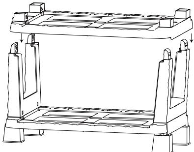
EN: Put the Support frame on the left & right frame of the support frame and confirm that it cannot be moved.
