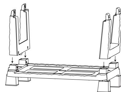
**EN:** Put the left & right frame into the bottom hole of the support frame and confirm that it cannot be moved.
