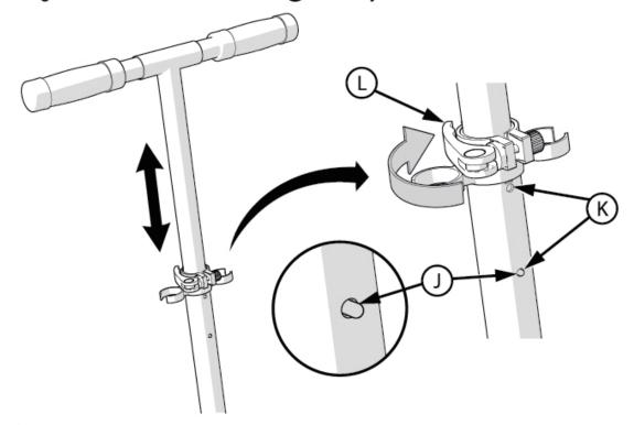
**WARNING:** The Quick Release Lock must be sufficiently tightened to hold the handlebar in place.
