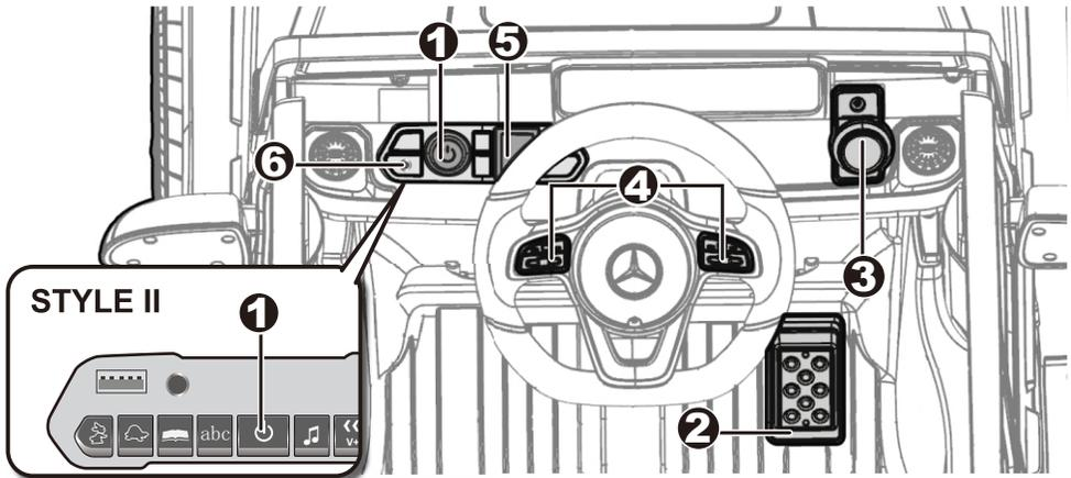
1. **Power button:** Turns the vehicle on and off.
