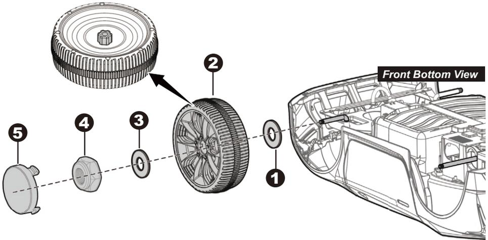
Remove all the parts from the front axle.
