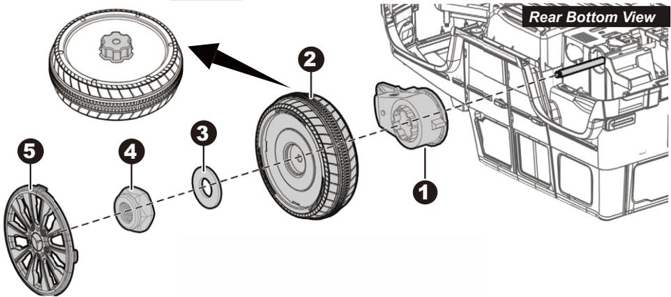
Remove all the parts from the rear axle.
