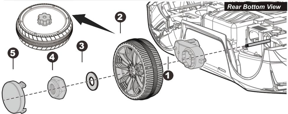
Remove all the parts from the rear axle.
