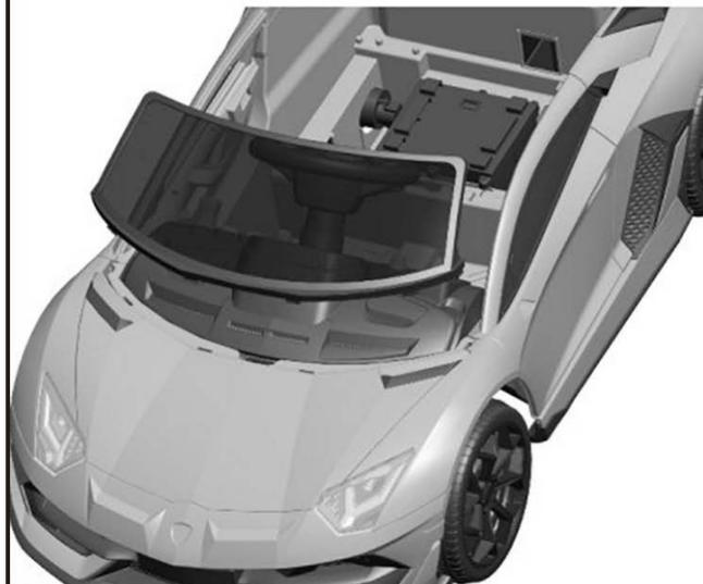
Fit the tabs on the windshield assembly into the slots in the body. Push the windshield assembly to "snap" in place. Make sure it fits securely.
