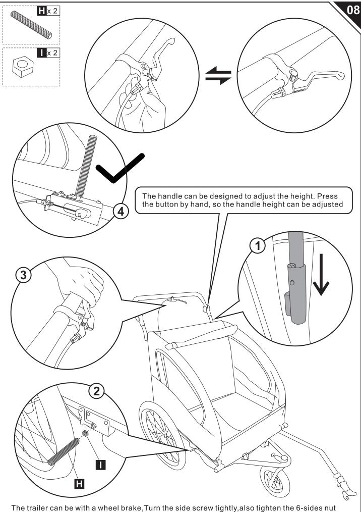
The trailer can be with a wheel brake, Turn the side screw tightly, also tighten the 6-sides nut with tools. Teh brake on the handle can control the wheel brake. When you close the brake on the handle bar and press down the screw , so the trailer can not go forward.
