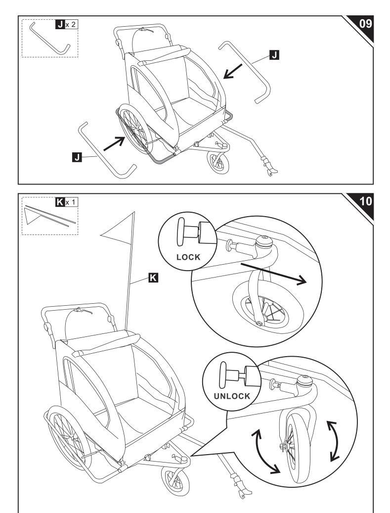
Black knob can control the wheel condition(lock Or unlock) Pull out and turn the black knob, the wheel position can be controlled.
