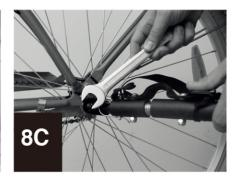
Remove rear wheel bolt. Attach quick release mounting bolt to the wheel. Re-tighten rear wheel bolt. Attach quick release pin to the trailer arm and latch securely. Figure **8A,8B** and **8C**.
