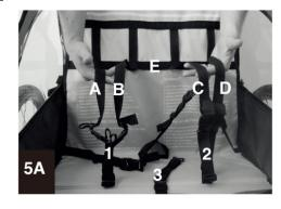
Disconnect the shoulder harness clips and the seat belt buckle. Place the children side by side on the seat. Place shoulder strap A over the first child's right shoulder and shoulder strap B over the first child's left shoulder. Place shoulder strap C over the second child's right shoulder and shoulder strap D over the second child's left shoulder.
