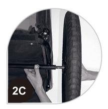
Lift the rear of the frame enough to allow you to insert the wheel axle into the hole in the side of the frame. Figure 2A.
