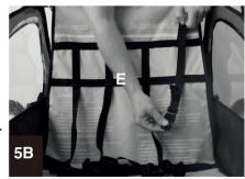
held snugly in place. The crotch straps should be adjusted so that the children do not slide too far forward. Make sure that the shoulder straps and crotch straps are snug and secure for the safety of the children and the stability of the trailer. Attach the seat belt across both childrens' laps.
