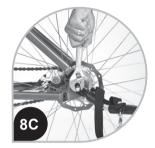
Remove rear wheel bolt. Attach quick release mounting bolt to the wheel. Re-tighten rear wheel bolt. Attach quick release pin to the trailer arm and latch securely. Figure 8A, 8B and 8C.
