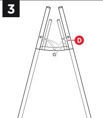
Loop the part D cord by alternating the cord through the holes and eyelets. Work your way around the circumference of the teepee and tie the cord together into a knot at the end.
