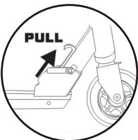
3. Pull the Lock Mechanism
