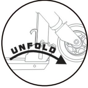
3. Unfold the Drive Bar tube
