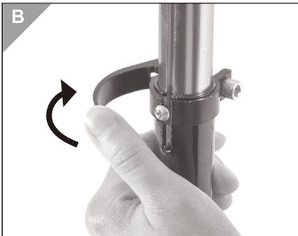
2. Press the metal pin on the steering column **2** and push the steering column to the desired height until the metal pin engages.
