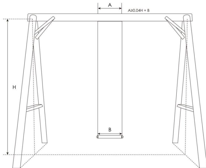
A. distance between the suspension points along the crossbeam. ( $A \geq 0.04H + B$ )
