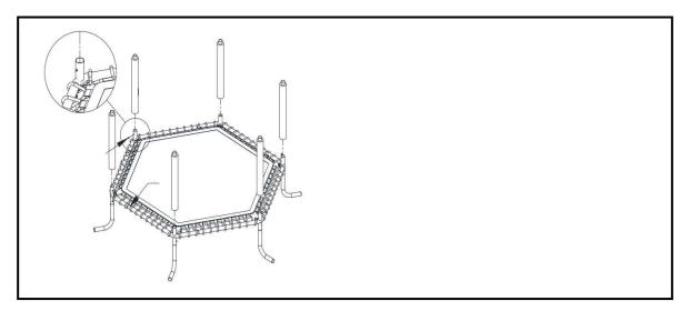
5. Secure the net from the top down to the main rack with the fastening buckle of the net on the ball head and tie the elastic band below to the pipe below.
