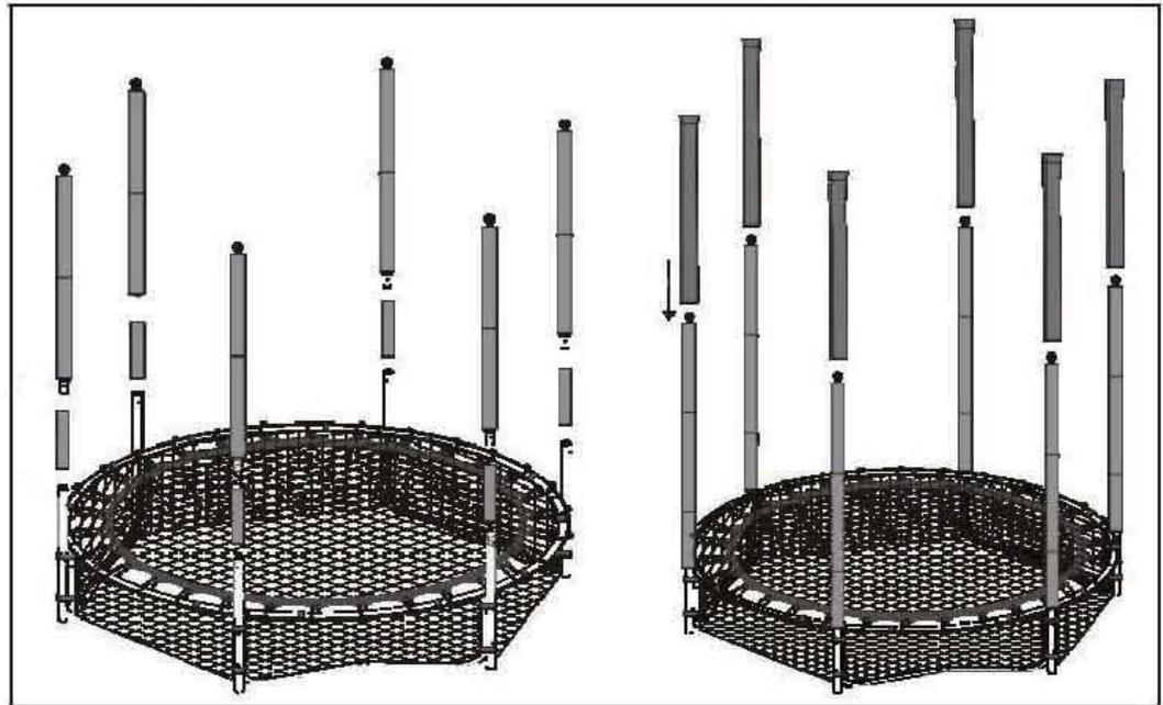
7. Secure the net from the top down to the main rack with the fastening buckle of the net on the ball head and tie the elastic band below to the pipe below.
