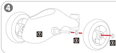
After the iron shaft passes through the main body of the bicycle, put into a hoop again, and then put through another wheel, and insert a hoop again.
