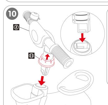
After assembling basket, push the big plastic ring up, and then plug the head of bike into body as picture showed. (Pay attention to the direction of the head and wheels, and turn the wheel to adjust the position, which corresponds to the position under the head of bike.)
