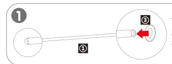
The two ends of the iron shaft are different. Put the hoop on the right side.
