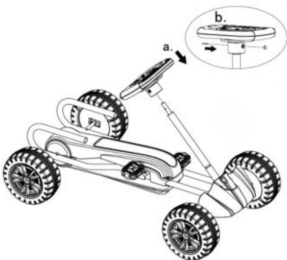
3. Place the steering wheel through the steering shaft and fix into place with M5\*40 screw, the lock into place with 5mm nut.
