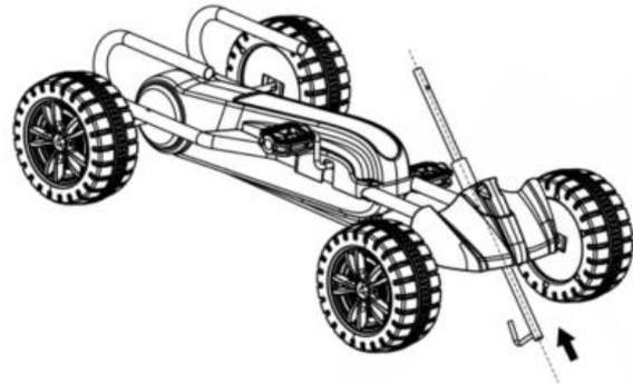
2. Put the Linear tube on the steering shaft.
