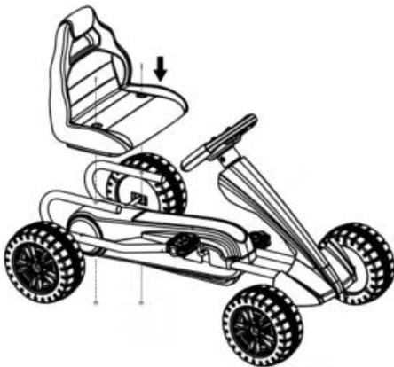
5. Fix the seat to the frame of the Vehicle using M5\*55mm bolts, ensure to use washers again where appropriate
