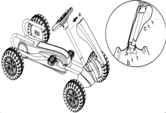
4. To fit the Panel to the frame ensure the 2 screw holes on Panel and frame are aligned. Tighten with M4\*10 screw.--b
