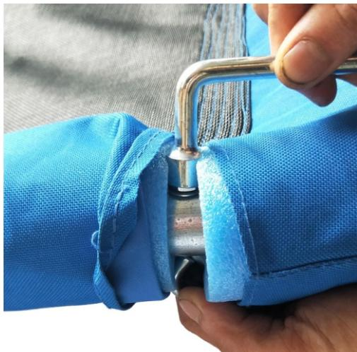
Tighten the bolt with screw nut (use the wrench included in the pack.)
