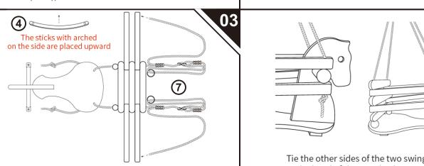
Use two swing ropes to separate one side, complete the connection of back wooden stick, side wooden stick, and wooden ball in sequence according to the figure, and then tie the horse base to tie it. (Keep the rope length consistent)
