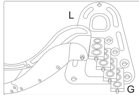
4. Install the slide plate and pedals on a slide side plate, and tighten the flower-shaped nut.
