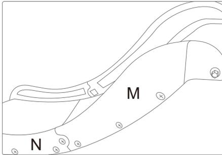
3. Install the slide length guardrail M, N to one side of the slide.
