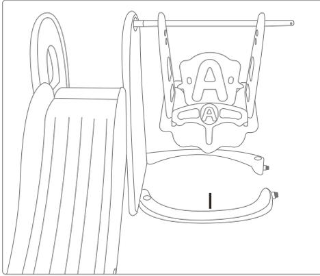
8. Install the swing base on the side plate of the slide.
