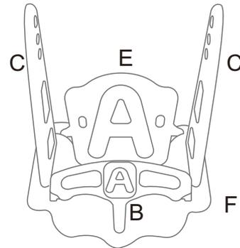
6. Install the swing backrest, swing side panels and swing armrests on the swing base and tighten the cross nut.
