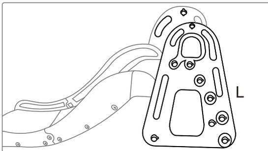
5. Install the corresponding hole on the other slide side plate and tighten the flower-shaped nut.
