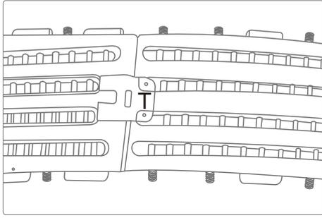
1. Connect the long slide plate and the short slide plate and tighten the iron screws.
