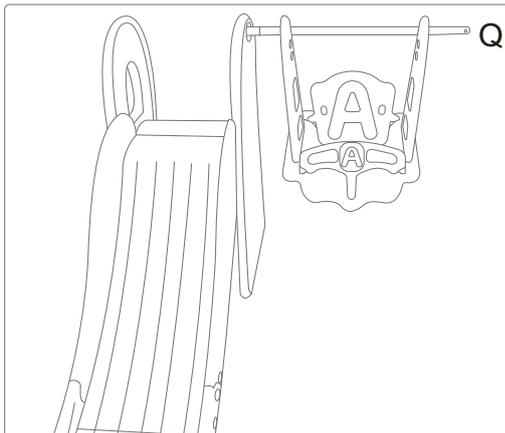
7. Install the spring buckle to the holes at both ends of the beam, pass through the swing side plate, fix it with the swing buckle, install the connecting buckle, and finally fix the slide side plate.
