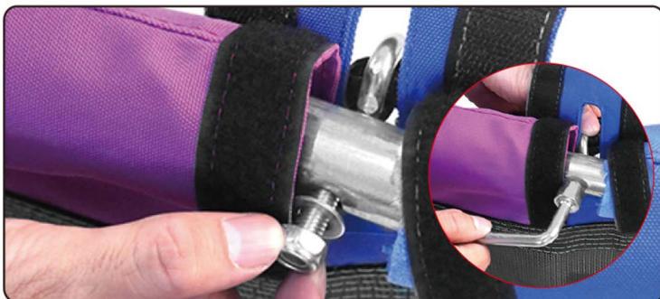
5. Put the spacers and nuts onto the bolts, tighten them with a wrench.
