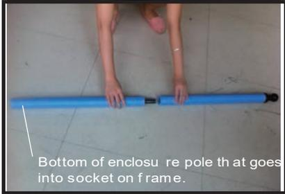
Bottom of enclosure pole that goes into socket on frame.
