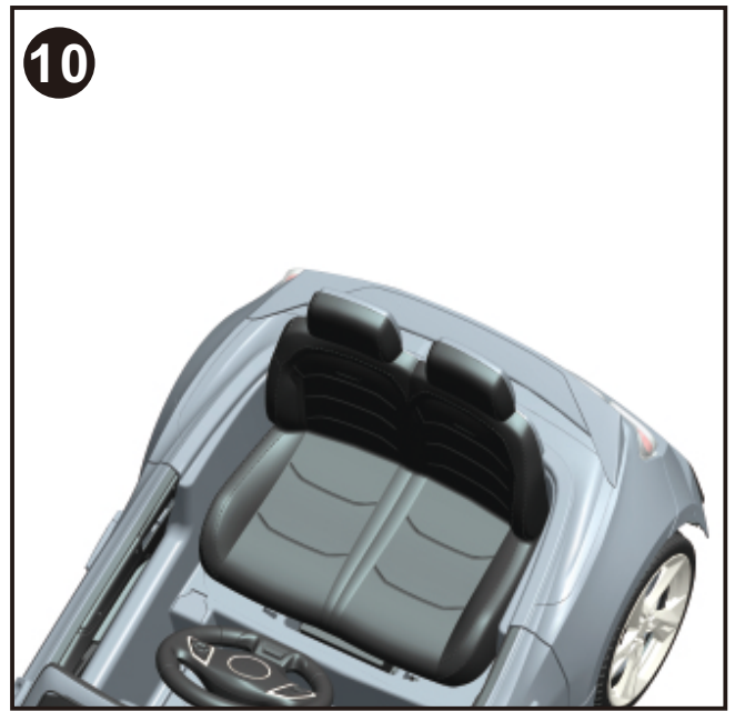
"Snap" the tabs on the seat into the slot of the vehicle.
