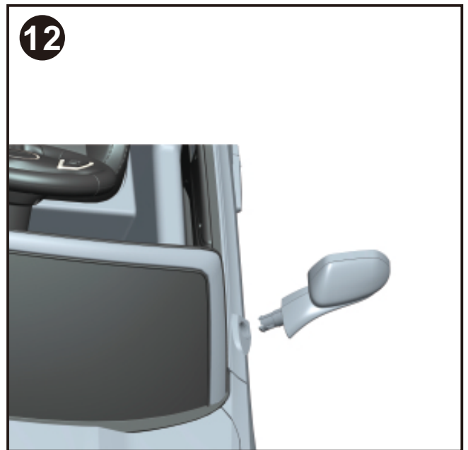
"Snap" the tab on the side mirror into the slot. Repeat the same procedures for the other side.
